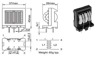
Recommended hole diameter: ø1.7 Dimensions in mm
